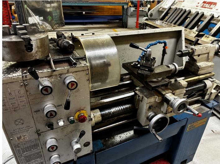
It includes all the safety features required for schools including chuck guard interlock and foot brake for emergencies.
