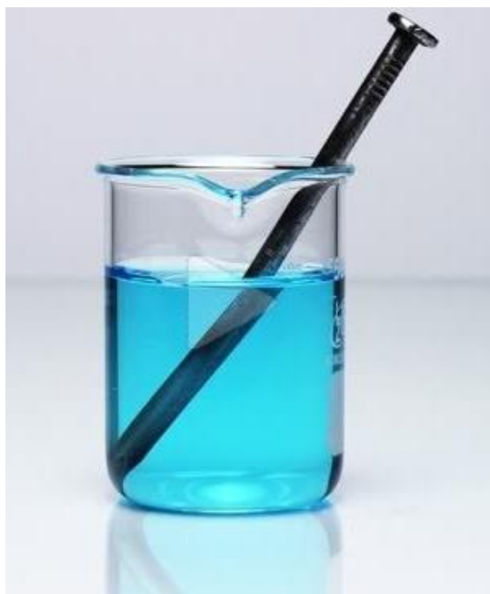
Reacting Iron with Copper sulphate
